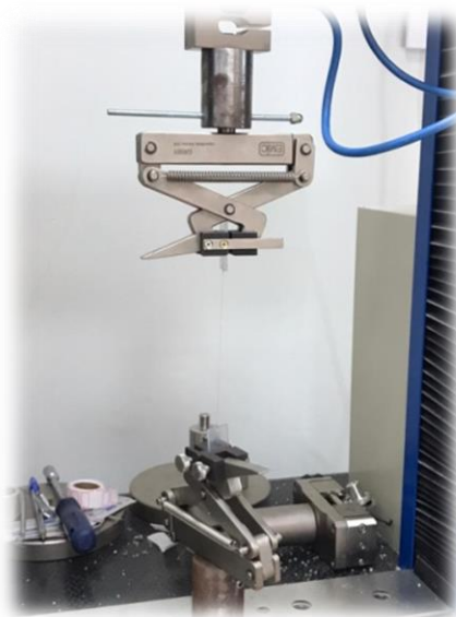
Fig. 6 – Sample positioned on the Universal Instron© testing machine
