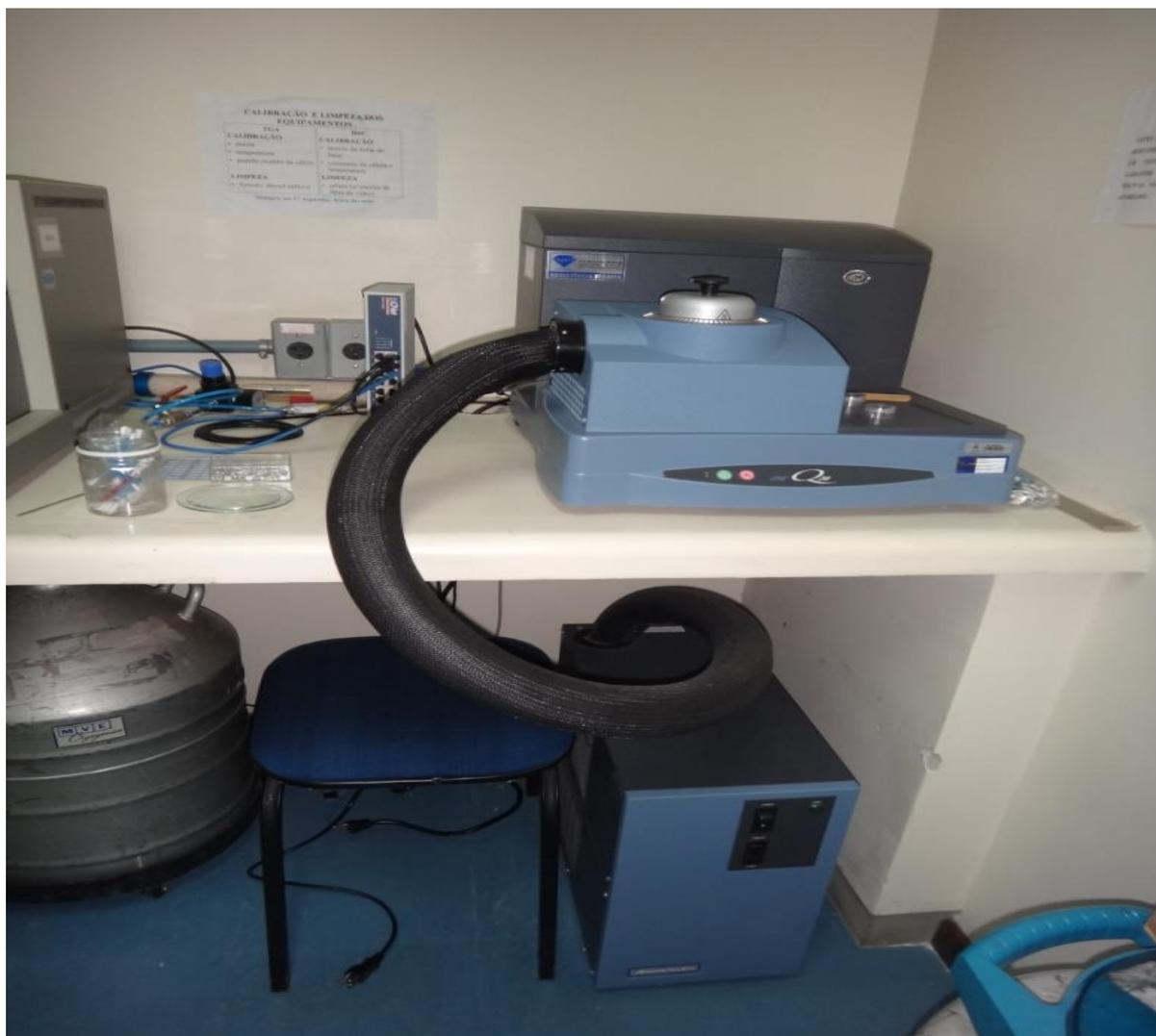
**Figura 7** – DSC Q20-TA Instruments.
